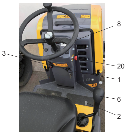
Figure. Instrument panel 1. Starter switch 2. Speed control 3. Parking brake 6. Forward/Reverse lever 8. Sprinkler knob 20. Emergency stop
