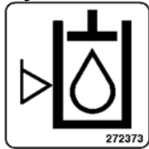
Hydraulic oil level
