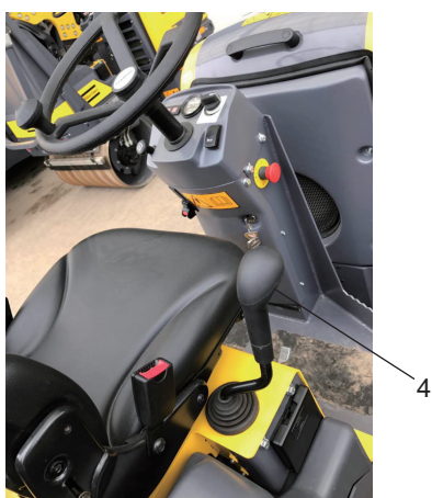
Fig. Forward/Reverse lever 4. Switch, vibration On/Off
