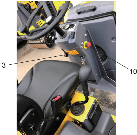
Fig. Controls 3. Parking brake 10. Emergency stop
