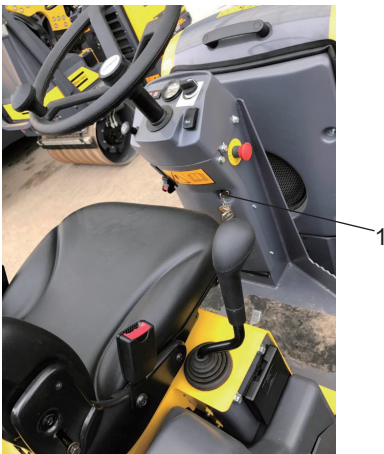
Fig. Instrument panel 1. Starter switch
