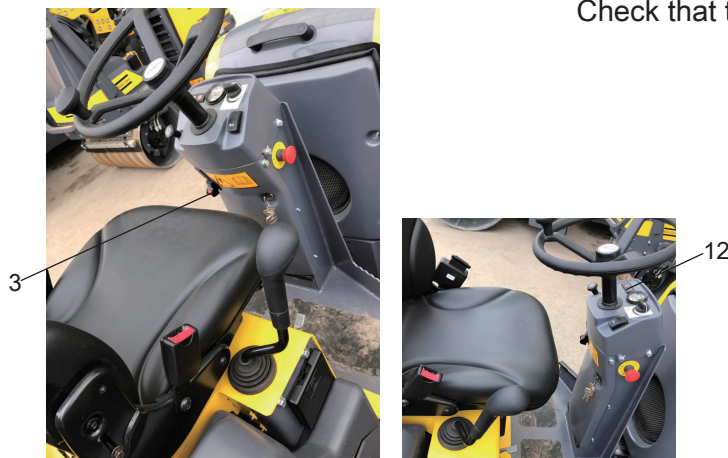
Figure. Control panel. 3. Parking brake 12. Parking brake warning lamp
